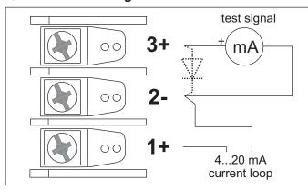
The 4...20 mA test can be measured without interruption of the low-potential circuit between terminal 3(+) and terminal 2(-). The output current is measured with an ammeter for mA across a diode in the output circuit.
