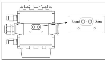
Below the type plate there are 2 key button for easy configuration of zero and span. The keys are Hall effect devices and are completely seperated from other parts of the enclosure.
