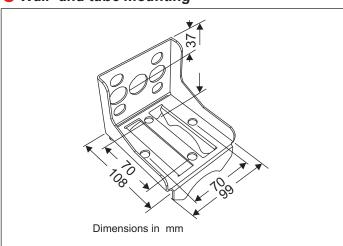
Holder made of steel (zinc coated) for mounting the device on walls or tubes is supplied with the device.
