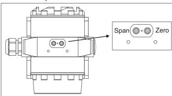
Below the type plate there are 2 key button for easy configuration of zero and span. The keys are Hall effect devices and are completely seperated from other parts of the enclosure.
