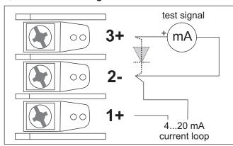
The 4...20 mA test can be measured without interruption of the low-potential circuit between terminal 3(+) and terminal 2(-). The output current is measured with an ammeter for mA across a diode in the output circuit.
